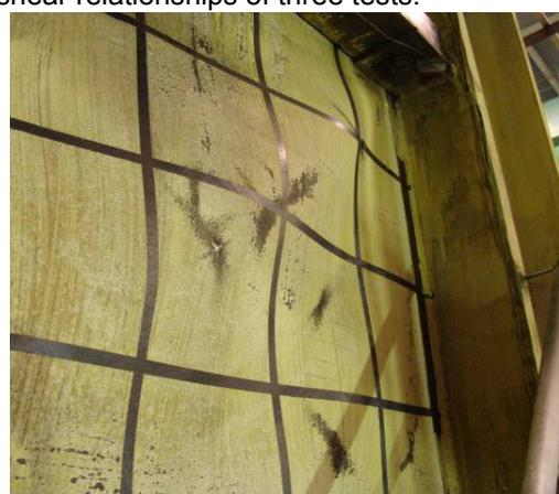
Photo 2. Steel plate buckling.
