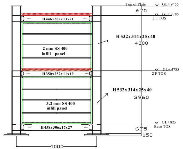
Figure 8. Specimen elevation.
