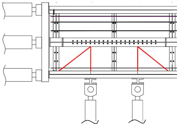
Figure 13. The arrangement of the actuators in a typical floor.
