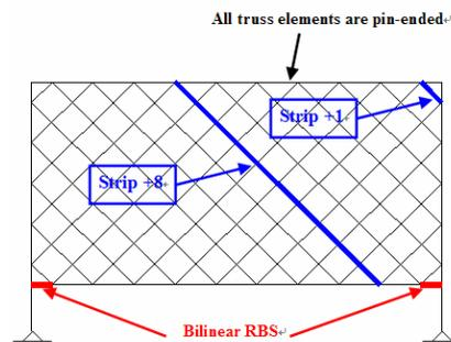
Figure 5. The SPSW specimen and PISA3D analytical model (Lin and Tsai, 2004).
