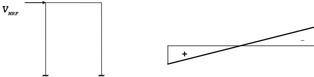
Figure 12. Moment diagram due to  $V_{\text{boundary frame}}$ .
