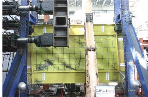
Figure 2. Tension field action.
