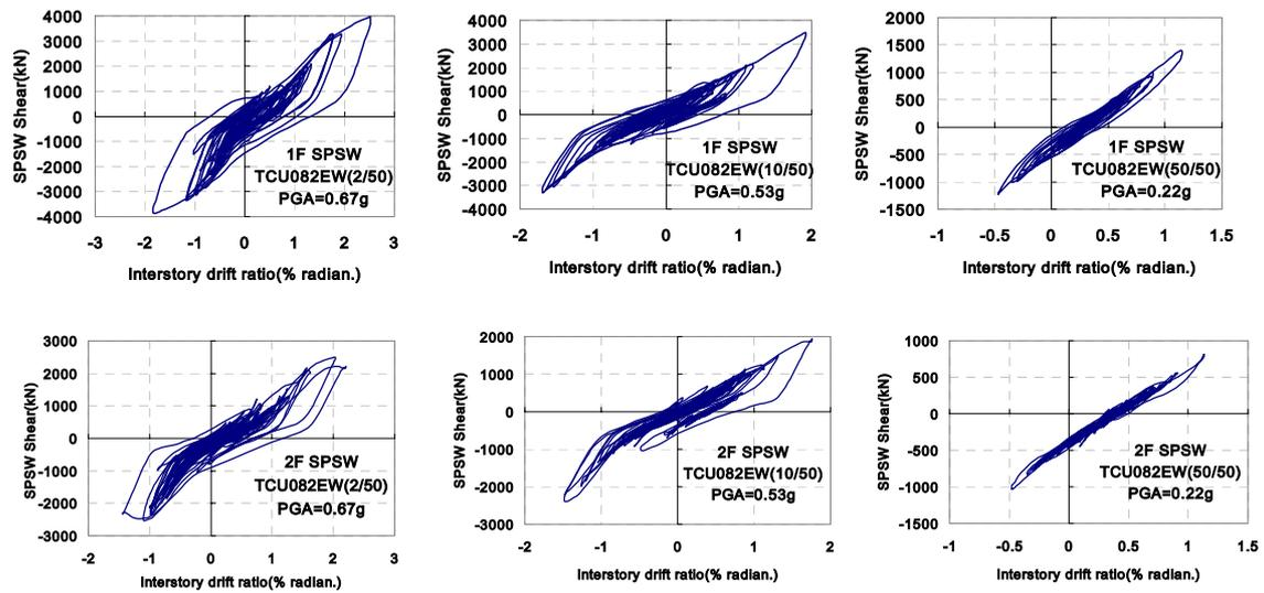
Figure 17. Inter-story drift ratio vs. story shear relationships of three tests.
