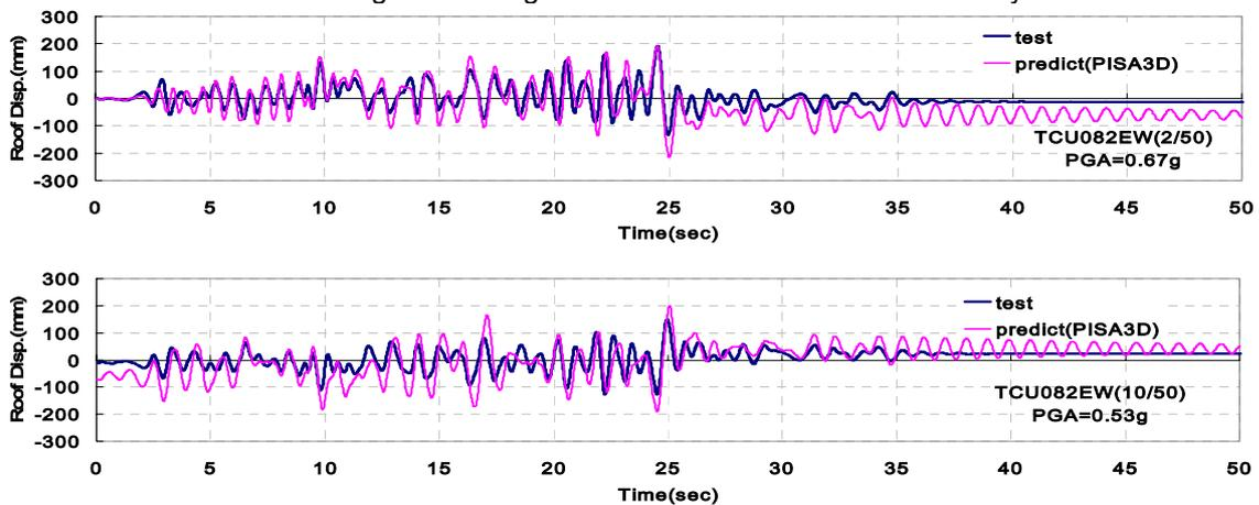
Figure 15. Roof displacement time histories (2/50&10/50).
