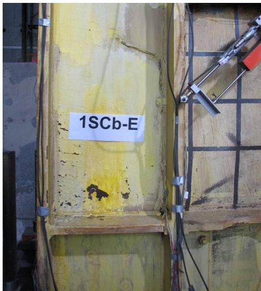
Photo 7. Column web yielding near the column base.
