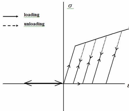
Figure 4. Tension-only material.
