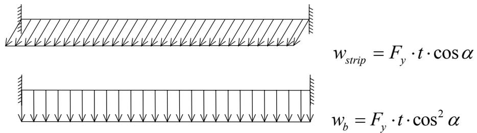
Figure 10. Beam boundary condition and distributed load.
