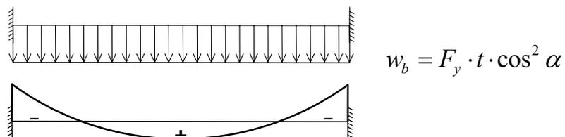
Figure 11. Moment diagram due to tension field.
