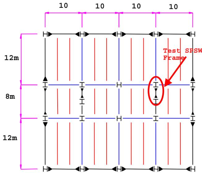
Figure 7. Floor framing plan of the prototype building.
